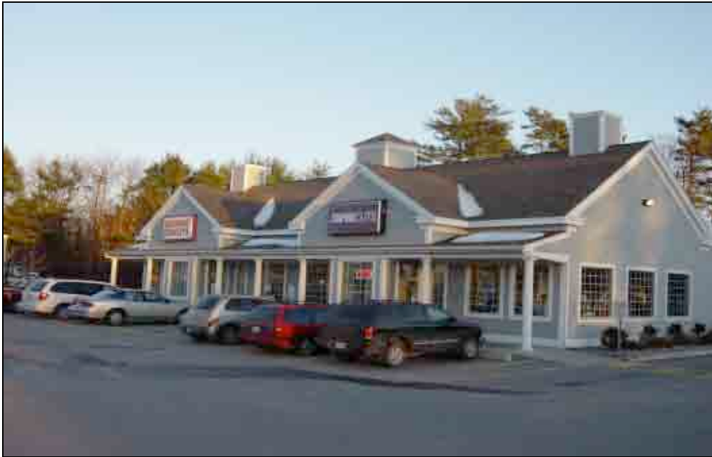
The shape and proportion of the roof shall be articulated so as to reduce the apparent size of new buildings and lend visual interest.
